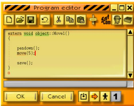
The exercise consists in tracing a 5 cm-long line on the ground. First use the following instruction to lower the pen:
