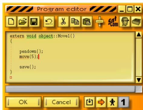
The editor works like any other Windows editor. The keywords of the CBOT programming language are displayed on a colored background, so that you can easily check the syntax. The automatic indentation according to the braces shows the structure of the program.
